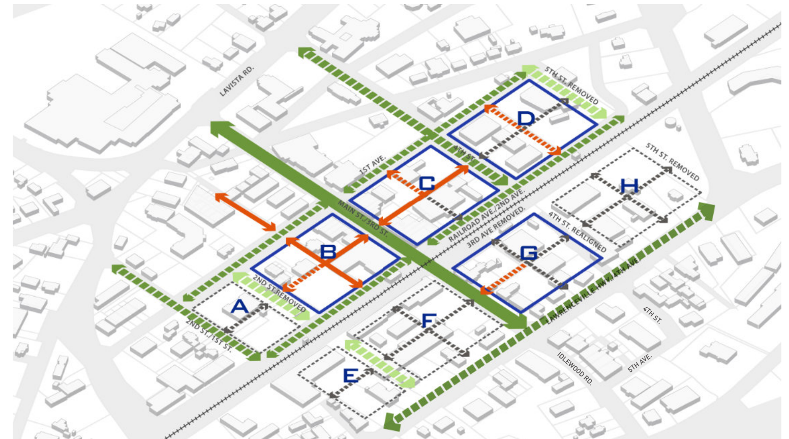
Preliminary Downtown Tucker Grid Analysis, comparison of 1891 grid with existing downtown block pattern
