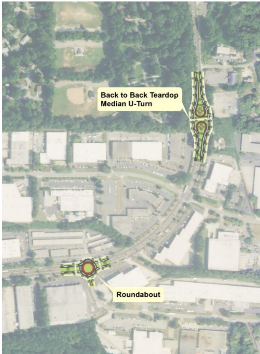
Figure 29: Mountain Industrial Boulevard and N. Royal Atlanta Drive/S. Royal Atlanta Drive Improvements
