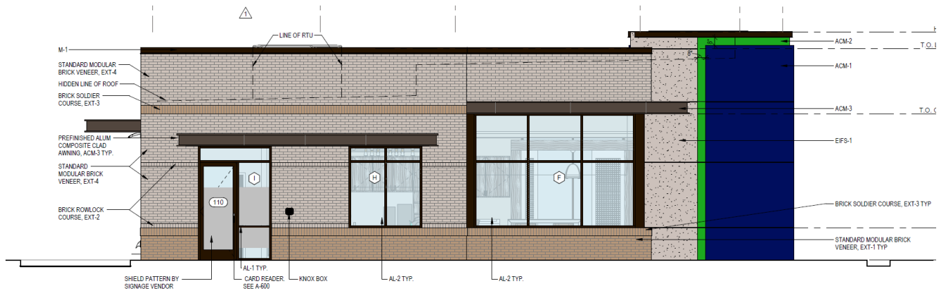
Figure 6. Montreal Road Elevation with 32.7% Fenestration.
