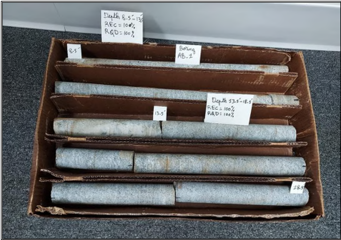
Rock Core from Boring AB-1 (1 st Run @ 8.5'-13.5', 2 nd Run @ 13.5'-18.5')
